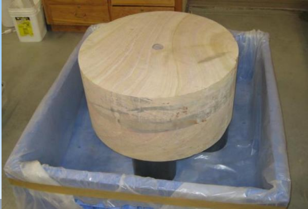
Figure 1a. Sandstone core (30-inch diameter) being extracted in Alabama. Figure 1b. Sandstone core undergoing hydraulic testing in the MSU laboratory.
